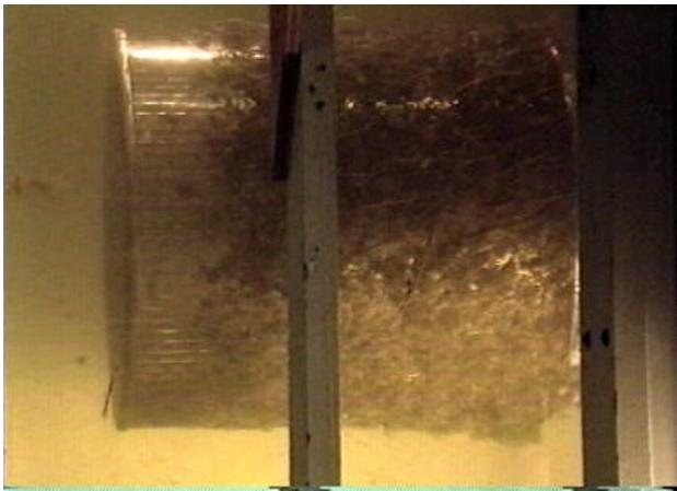
**Figure 3** - Debris loading on the screen after about 2 hours operation. The partially plugged screen shows little debris loading on the upstream end of the screen.
