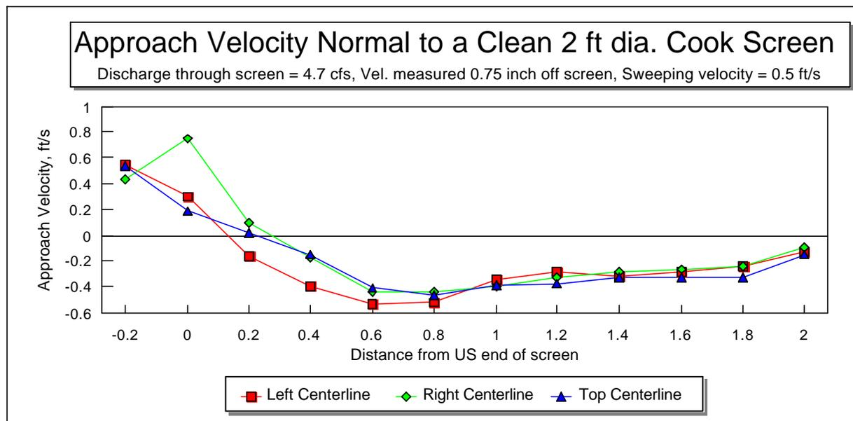
**Figure 2** - Velocity profile normal to a clean screen.
