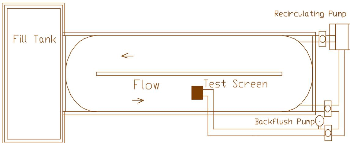
Figure 1 - Layout of Fish Screen Test Facility
