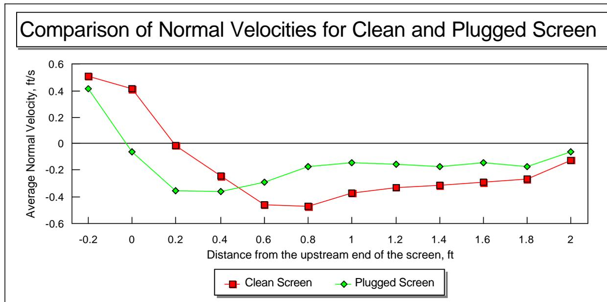
**Figure 6** - Comparison of approach velocities normal to the screen for clean and plugged conditions.
