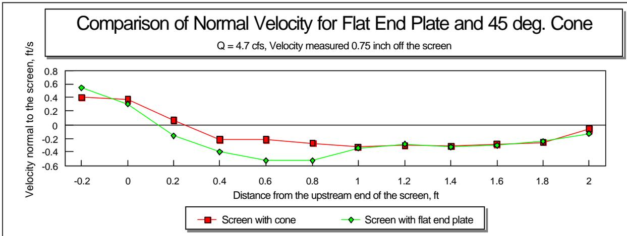
**Figure 11** - Comparison of approach velocity normal to the screen for a flat end plat and a 45 degree end cone.
