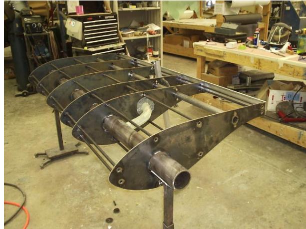
Figure 6: Model internal construction details.
