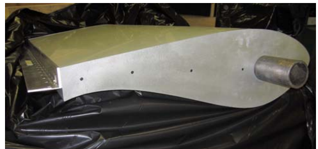
Figure 8: Flatback wind tunnel model with splitter plate attached.
