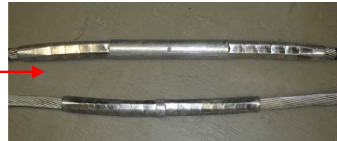
Compression splice connector fittings: (top) the two-stage fitting (TSC), (bottom) the single stage fitting (SSC).
