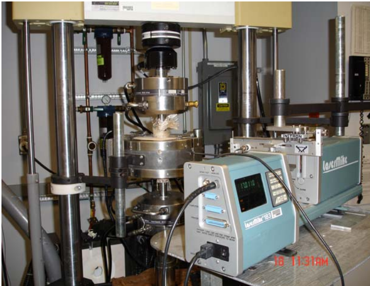
High temperature tensile test with the associated deformation control set-up.
