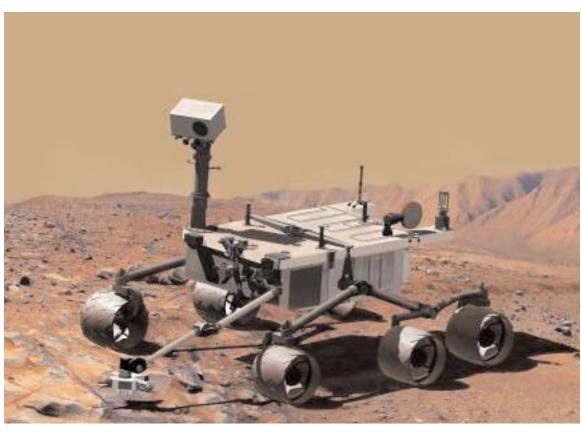
ing NASA space shuttles. During the 3 minutes before touchdown the spacecraft would slow its descent with a parachute, then use retro rockets mounted around the rim of an upper stage for the final 500 meters (1,640 feet) of the descent. In the final seconds, the hovering upper stage would act as a sky crane, lowering the upright rover on a tether to the surface.
