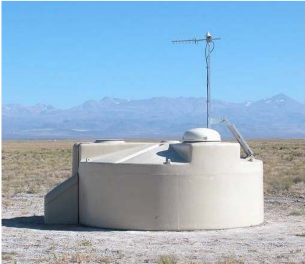
Water Cherenkov measures EM + 25x muons
