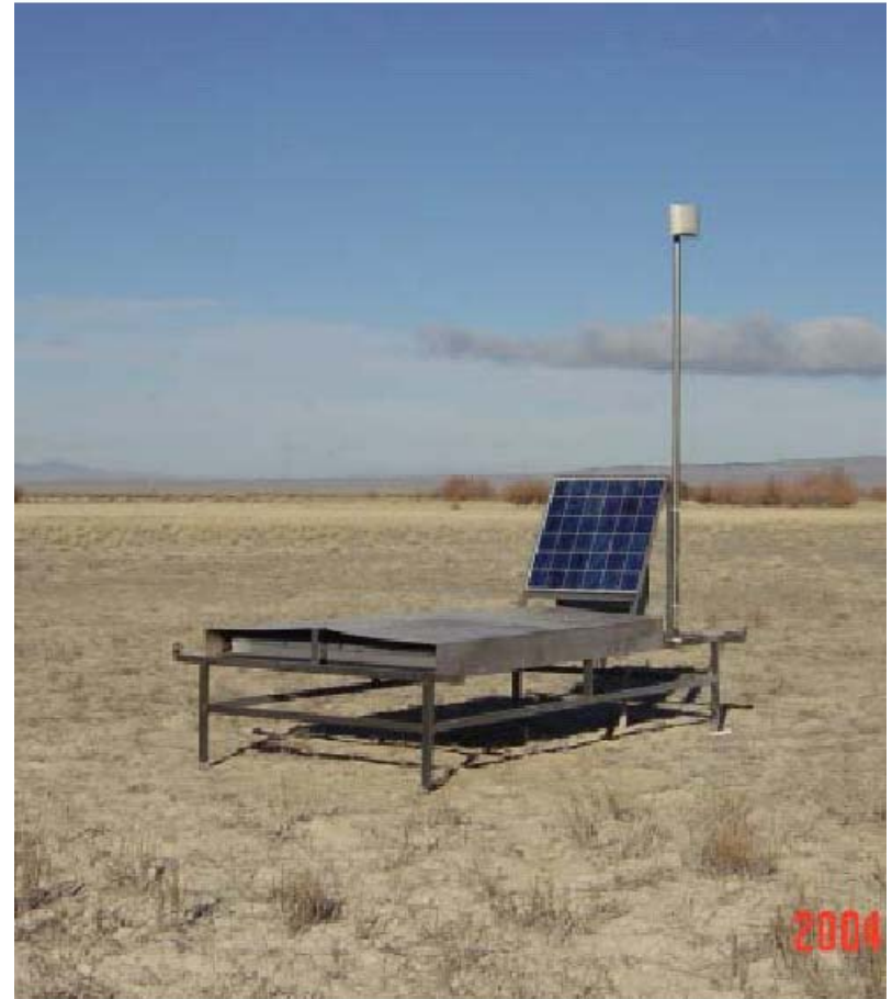
Unshielded scintillators measure mainly EM.
