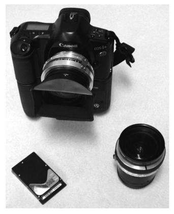
FIG. 2. Kodak DCS1m with Leica 19 mm lens mounted and Schneider 28 mm lens in the foreground. Images are saved on PCMCIA cards. Metal rings were fitted around both lenses to fix the focus distance and allow calibration for different reproducible distance settings.
