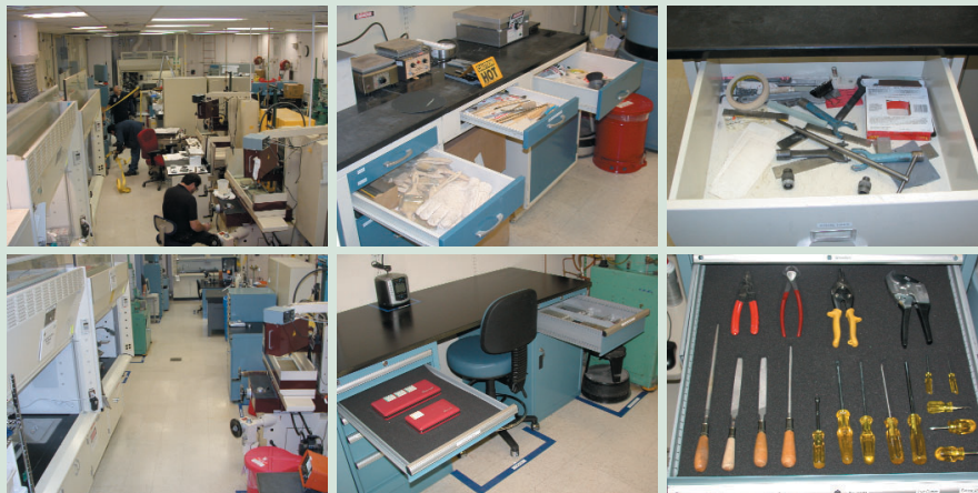
Before (top) and after (bottom) pictures show the 6S difference at three levels. Left, the overall workspace is spacious, organized and uncluttered. Center, new workstations are functional and ergonomic. Right, hand tools are organized and easy to find.
