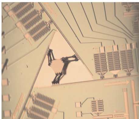
An XYZ MEMS device attached to three LSTD's is shown popped-up above the fabrication plane. The platform is 230 microns across.
