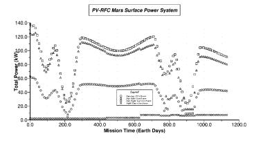
Figure 6. PV Array and User Power
