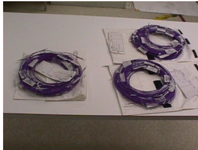
Terminated Flight Links (QTY 36 in 12 Configurations stored In four different low level softpacks)
