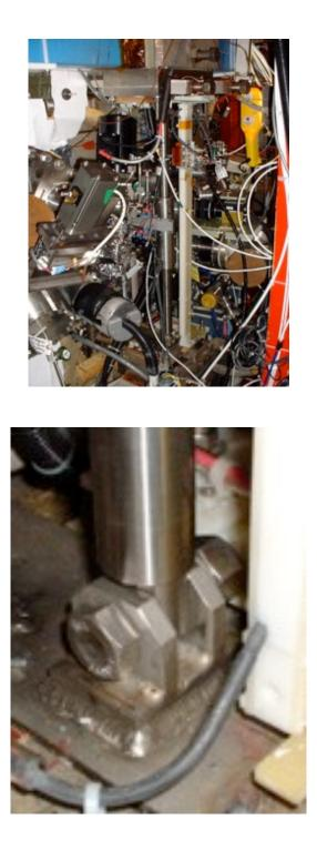
The strut is necked down to a cross section of approximately 1" x 3/4" where it engages the clevis and shear bolt which is 3/4" diameter. Thickness of clevis fingers are 1/4".
