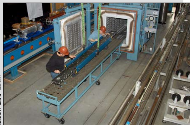
On the Bldg. 902 production floor, Tom van Winckel and Glenn Jochen, Superconducting Magnet Division, prepare to "bake" a magnet coil of niobium (Nb) and tin (Sn) in a huge oven to produce the superconducting compound Nb_3Sn being tested at BNL for use in a future upgrade to the Large Hadron Collider in Switzerland.
