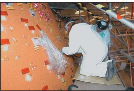
Inside the Vehicle Assembly Building at NASA's Kennedy Space Center, Fla., United Space Alliance technicians Brenda Morris and Brian Williams repair a hail-damaged area on Space Shuttle Atlantis' external tank. In late February, the tank received hail damage during a severe thunderstorm that passed through the Kennedy Center Launch Complex 39 area, leaving divots in the giant tank's foam insulation.
