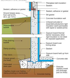
**Figure 13** Full height basement insulation
