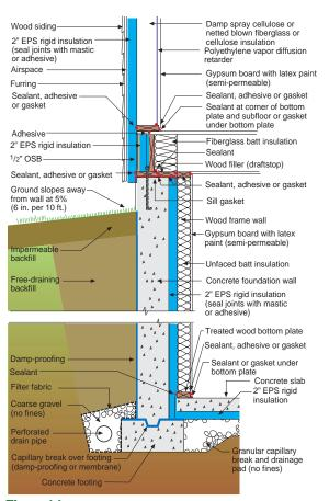
**Figure 14** Additional interior basement insulation
