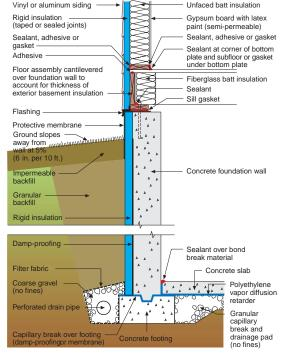
**Figure 10** Exterior basement insulation
