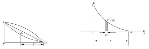
Fig. 2 Expression of even slope, concave slope and convex slope
