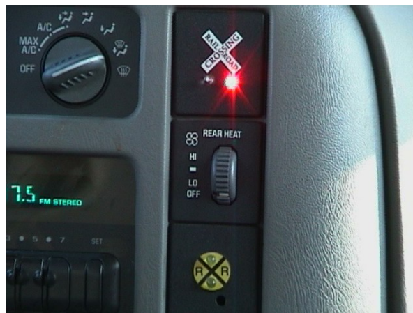
Figure 24. Minnesota Guidestar In-Vehicle Warning System [10]
