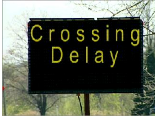
Figure 8. Long Island Railroad Intelligent Grade Crossing Variable Message Sign on Roadway in New Hyde Park, NY [10]
