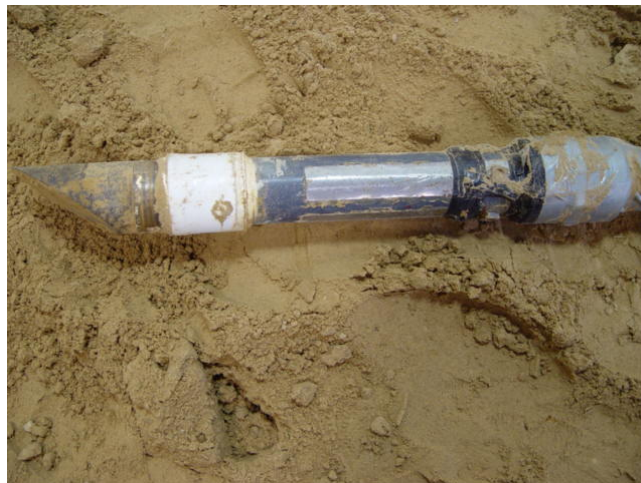
Figure 13. Close-up Of Prototype With Steel Shim Sense Elements
