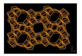
ZSM-5 on Oxide Coated SS Good intercrystalline growth ≈ 7microns thick
