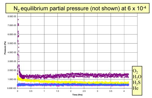
H<sub>2</sub>S does not permeate thru defect-free ZSM-5 membrane. No short term damage
