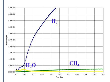
50/50 H<sub>2</sub>/CH<sub>4</sub> flowing thru defect free Silicalite "Zoom in" on H<sub>2</sub>O partial pressure
