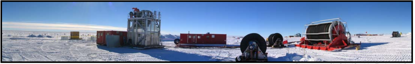
The IceCube drill, deployment tower and hose assembly ready to be put to use at the South Pole.
