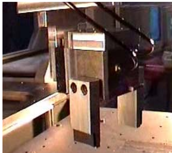
Figure 48 J-box pick-and-place end-effector.
