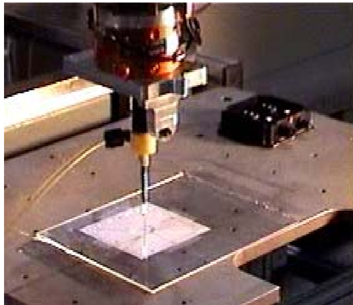
Figure 45 Alcohol dispense end-effector.
