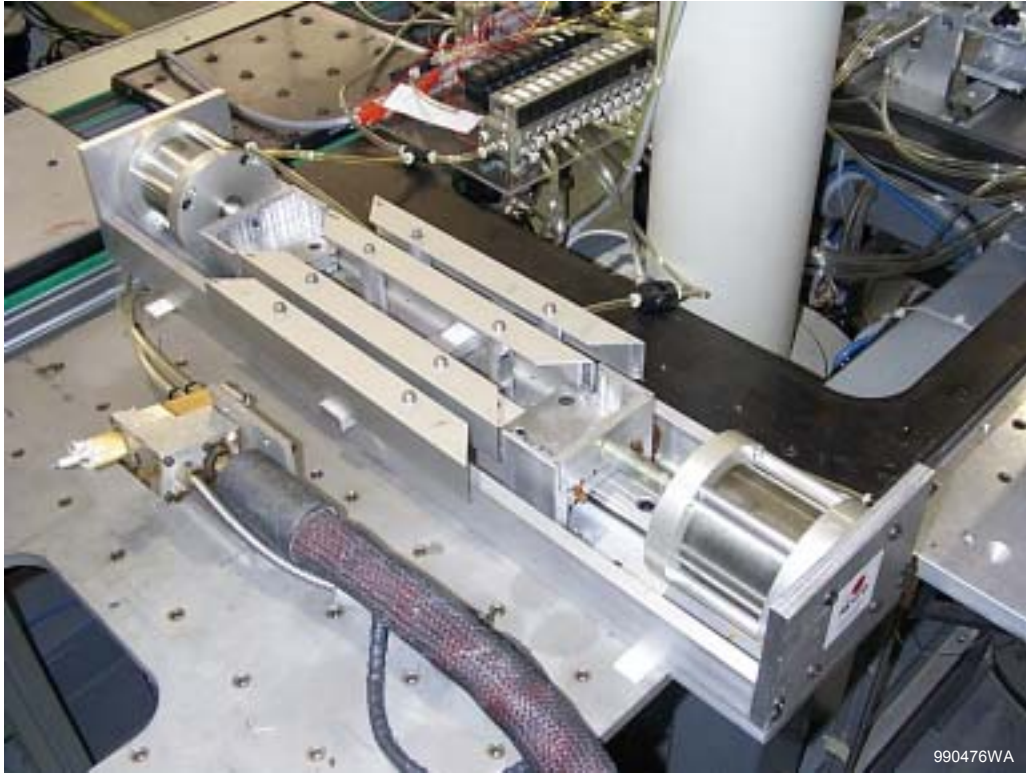
Figure 12 Prototype corner key inserter (center) and sealant dispense head (left).
