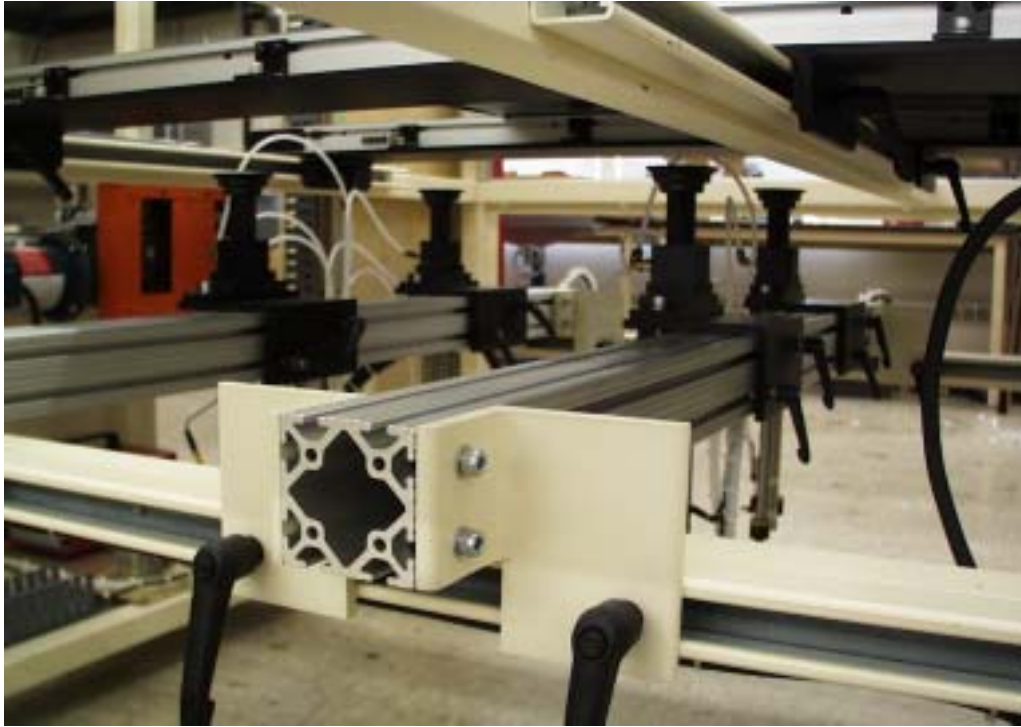
Figure 33 Module vacuum lift, retracted under belt conveyors.
