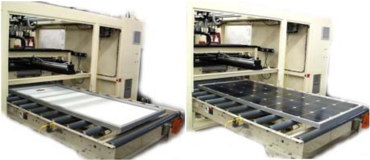
Figure 42 Module sealed and framed automatically, on the output conveyor of the SPI-FRAME 350. Module is processed facedown, as shown at left. Module is shown face-up at right.
