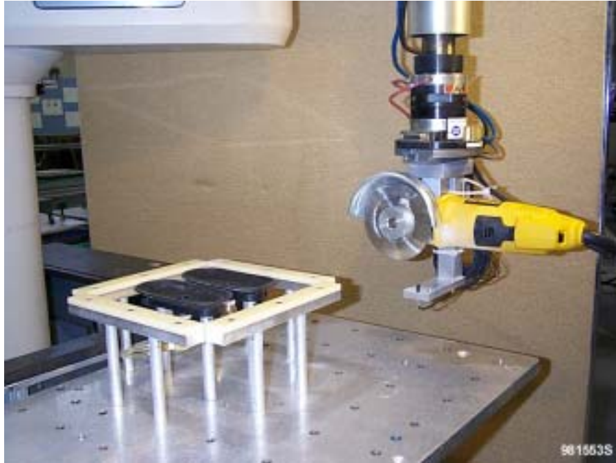
Figure 8 Spinning saw prototype setup for module trimming.
