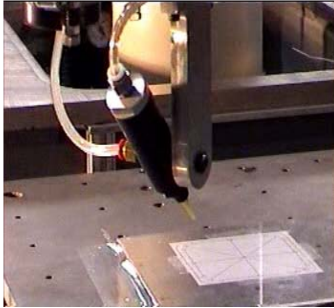
Figure 46 Sealant dispense end-effector.
