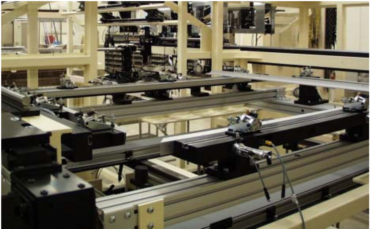
Figure 39 Two-axis frame press.
