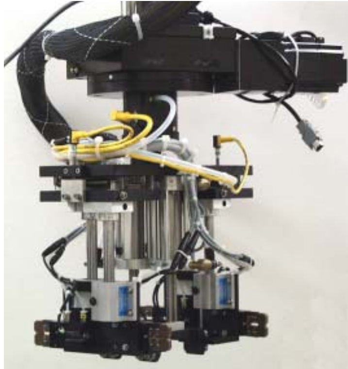
Figure 40 Framer robot end-effector.
