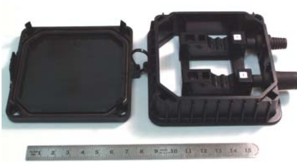
Figure 44 Multi-Contact junction box, model PV-JB/2-UR, with cover open (scale is in cm).
