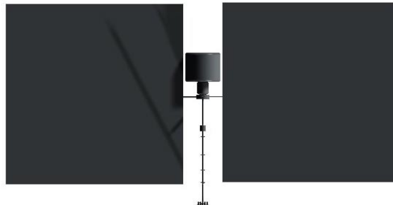
Figure 5. Lunar Gateway SEP Transfer Vehicle. PV arrays shown to scale; Hall thruster pallet shown at the bottom of the illustration, and the payload mass is the approximately square element shown attached to the base pallet near the center of the image.
