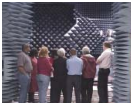
Compact Range Antenna Measurement Chamber
