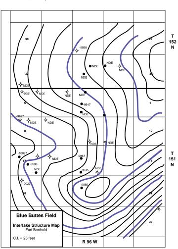
Figure FB-12.3. Structure contour map of Interlake interval, Blue Buttes Field. Shows anticlinal nose development with production located somewhat off structure. This indicates a strong stratigraphic component which assists trapping mechanism.
