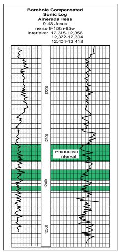
Figure FB-12.2. Example of wireline log through Silurian interval in Blue Buttes Field.
