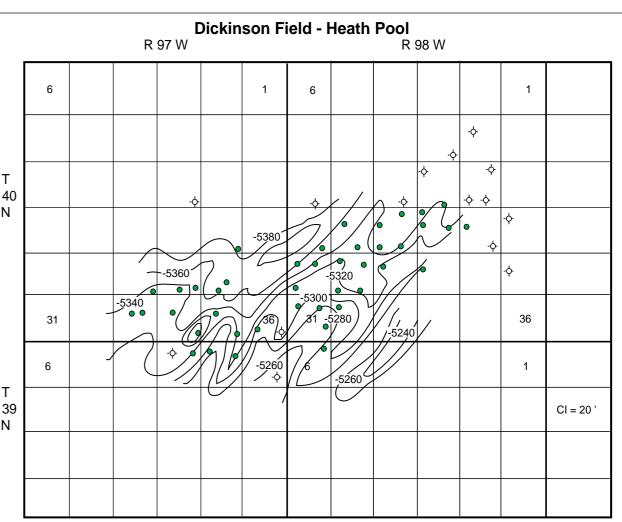
**Figure FB-13.2.** Structure map of Dickinson Field, top of Heath. Complex structural configuration reflects the depositional patterns associated with fluvial, deltaic and nearshore marine environments (after Williston Basin Field Summaries, 1984).
