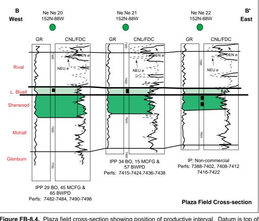
Figure FB-8.4. Plaza field cross-section showing position of productive interval. Datum is top of Sherwood horizon (after Sperr et al, 1993).
