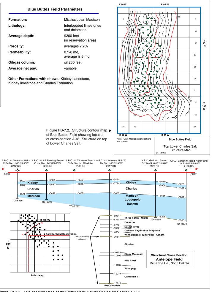
Figure FB-7.3. Antelope field cross-section (after North Dakota Geological Society, 1962).
