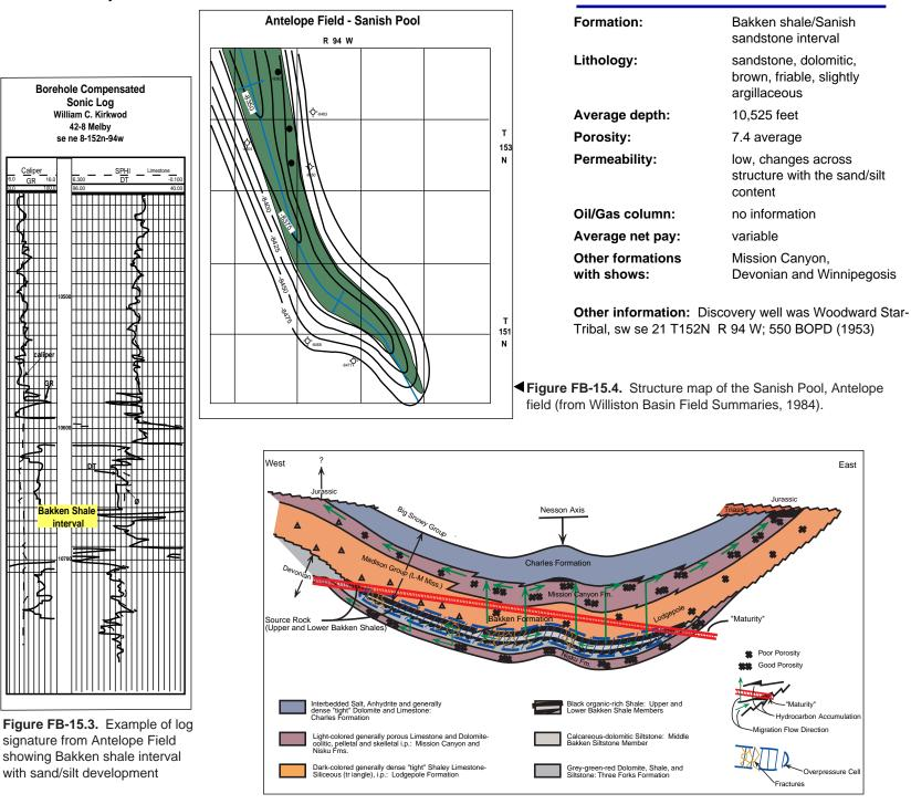
**Figure FB-15.5.** Schematic east-west section across the Williston Basin showing source-rock maturity, fluid over-pressure, fracture, migration and hydrocarbon accumulation patterns in the Bakken formation and adjacent units (after Messiner, 1984).
