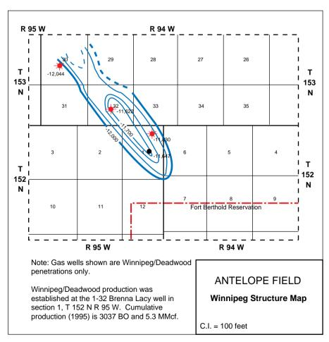
Figure FB-14.2. Structure contour map of the Winnepeg Fm., Antelope Field. Shows Winnepeg production correlated with anticlinal fold trend to the southeast.
