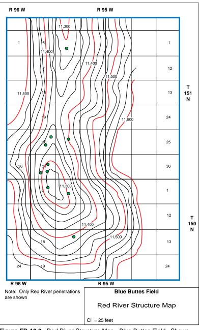
Figure FB-10.3. Red River Structure Map - Blue Buttes Field. Shows trend of Anticline development and production.
