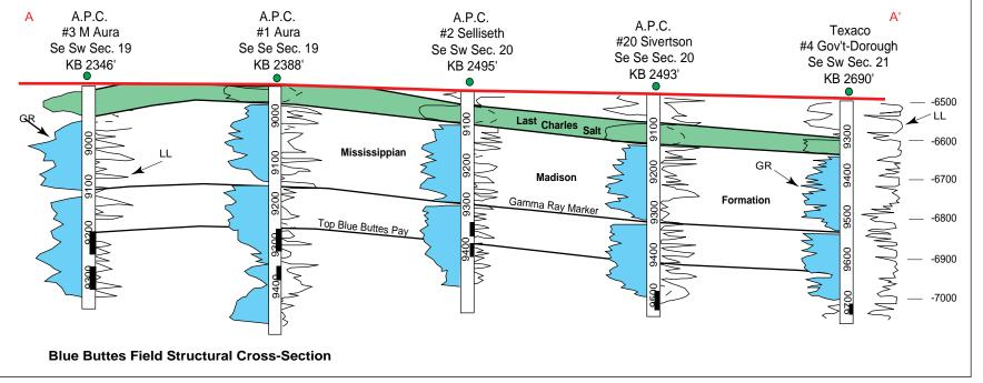
Figure FB-7.1. Blue Buttes Field structural cross-section (after Connelly, North Dakota Geological Society, 1962).
