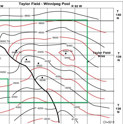
Figure FB-14.4. Taylor Field, Winnipeg Structure. Production strongly correlated to major fault with associated anticlinal nose development to the northwest (from Williston Basin
