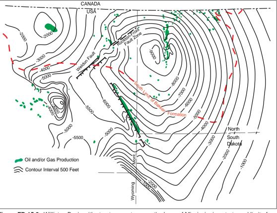
**Figure FB-15.2.** Williston Basin with structure contours on the base of Mississippian strata and limit of Bakken Formation (after Webster, 1987).
