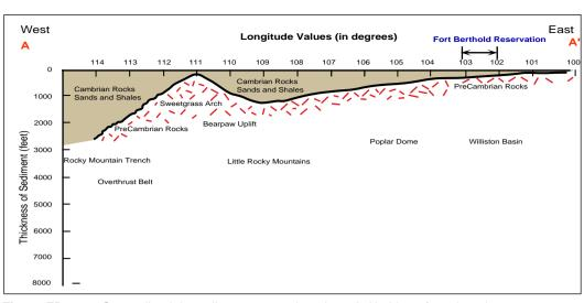
Figure FB-2.2. Generalized time-slice cross-section along A-A'. Line of section along 48 degrees latitude with selected points every 1 degree longitude. Datum is base Ordovician.
