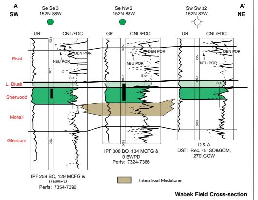
**Figure FB-8.3.** Wabek Field cross-section showing position of productive interval. Datum is top of Sherwood horizon (after Sperr et al, 1993)).
