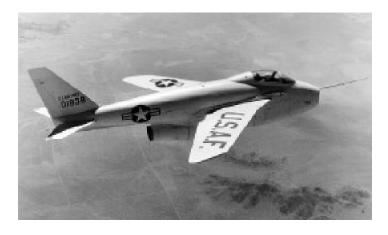
20 to 60 degrees at subsonic and transonic speeds. Results from these tests provided some of the design background for the F-111 and the Navy F-14 tactical aircraft.
