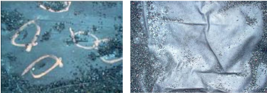
Figure 6-2. Examples of Perforated (left) and Intact (right) Liners
