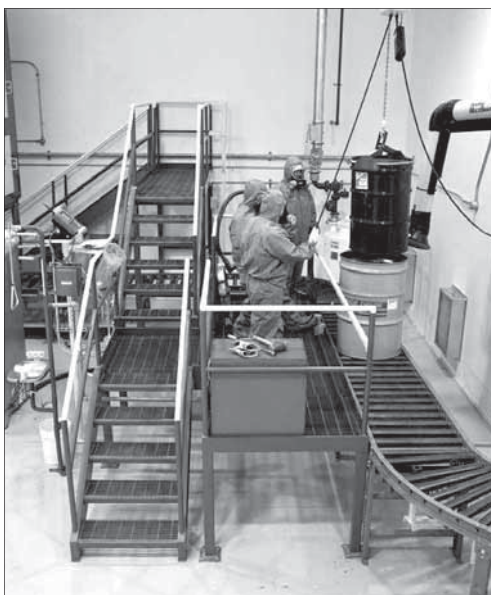
Workers package material at the Foster Wheeler TRU waste processing facility in Melton Valley.
