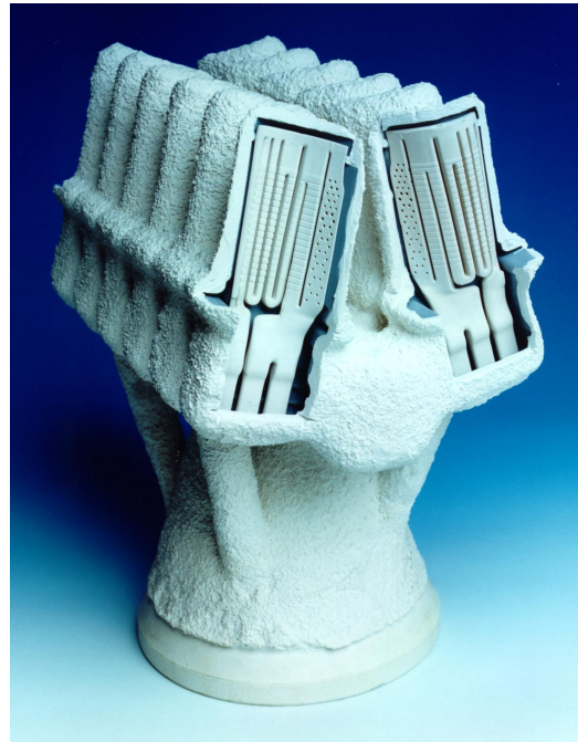
Fig. 8.10. Investment casting mold cut away to show a core inserted in the interior of one of the gas turbine engine blade mold cavities.
