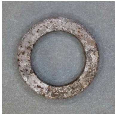
Mild Corrosion (Test #6)
