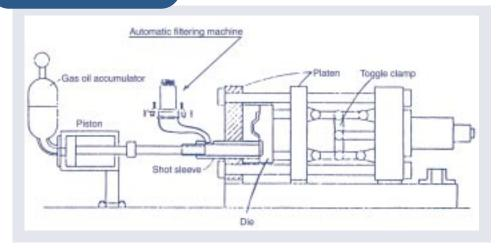
This schematic shows where an automatic filtering system would be installed where molten metal enters the die of one of the most common die casters. These types of die casters are used to produce many aluminum and zinc castings such as automobile parts and tools.
