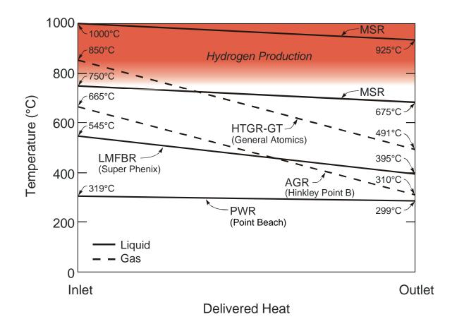
Delivering Heat at Nearly Constant High Temperature Allows Use of Advanced Electric Power Cycles
