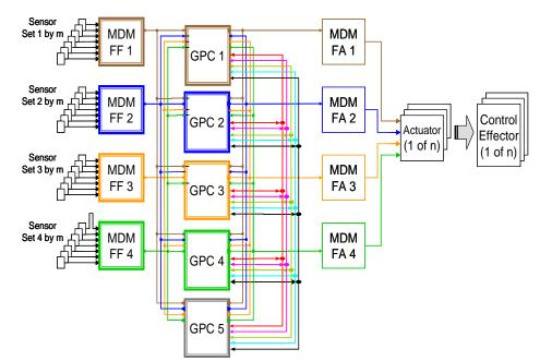
A much simpler and strait-forward redundancy management system for future architectures is necessary to be cost effective
