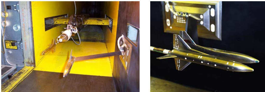
Fig. 6. Photographs of the LBGG Configuration Installed in Test Section 2 of the NASA LaRC UPWT.
