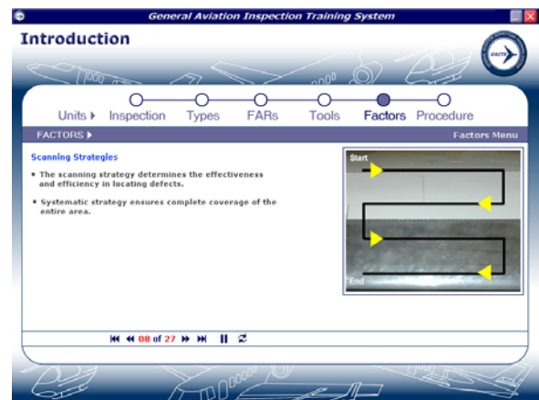
Figure 1: The Introduction Module demonstrates inspection procedures, such as a systematic search strategy
