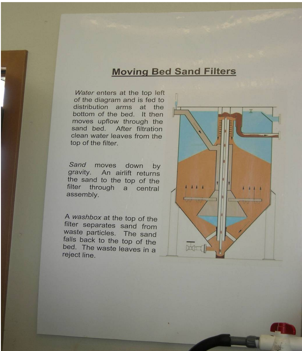
Cutaway diagram of Centra-Flo filter at Blue PRO installation at Hayden HWRF
