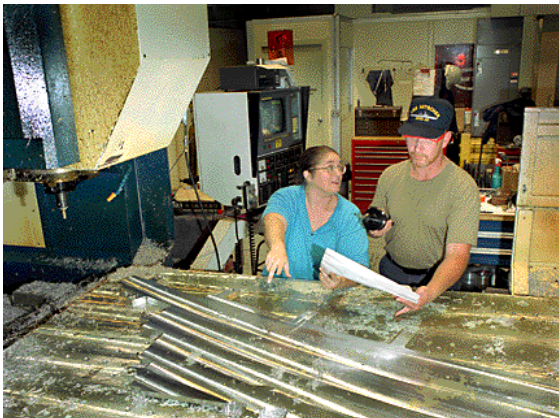
Elisabeth Deazley and Edward Losee, both of BNL's Central Shops Division, inspect a component of an exit chamber being manufactured in Central Shops as part of an upgrade to the x-ray ring at BNL's National Synchrotron Light Source (NSLS). The upgrade, which will result in a more intense beam, will cause an increase in temperature in the ring. Three new exit chambers will compensate for the heat increase. Over 12 feet long when assembled, the chambers must be constructed to an exacting five-thousandths of an inch tolerance. The first chamber will be incorporated into the ring in December.
