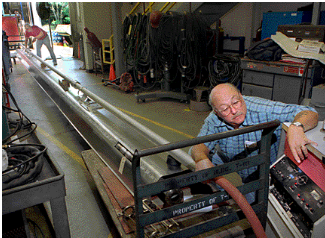
Sheet Metal and Welding Supervisor Al Farland (front) and Gene Sorensen, both of BNL's Central Shops Division, are conducting a vacuum leak check on a tube from a lower heat shield of a RHIC magnet. The beam pipe in which RHIC's ions travel is visible slightly below and to the left of Farland's right hand. This type of evaluation is an example of Central Shops' nondestructive, on-site testing capability.
