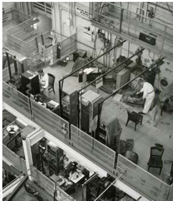
The west face of the Brookhaven Graphite Research Reactor in 1962, showing some of the experimental installations. At this face, there were 30 separate holes through the shielding wall that could accommodate different experiments.
