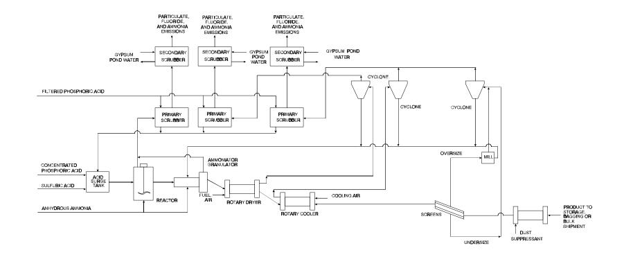
Figure 8.5.3-1. Ammonium phosphate process flow diagram.
