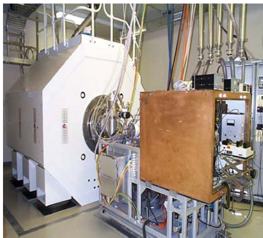
Figure 2. Wide-bore, passively shielded 11.5-T FTICR mass spectrometer.
