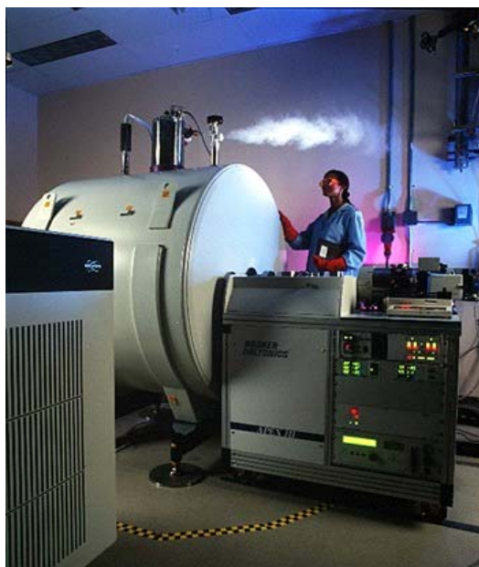
Figure 3. 150-mm bore, actively shielded 9.4-tesla FTICR instrument.
