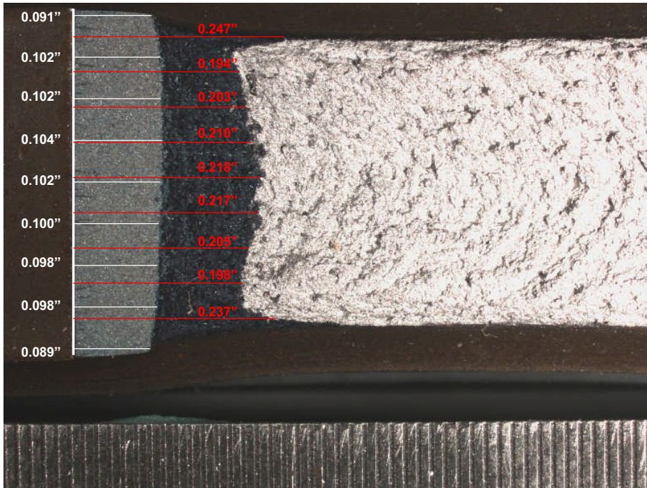
Figure A-10. Crack length measurements for specimen A4 (parent 90°) of the A516 steel
