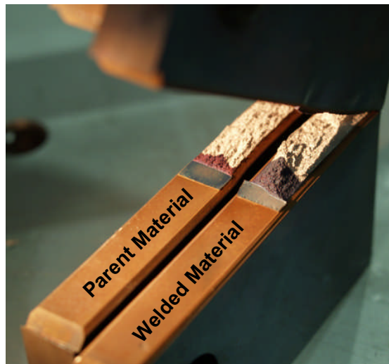
Figure 12. Photograph of the fracture surface of a pulse MIG weld.
