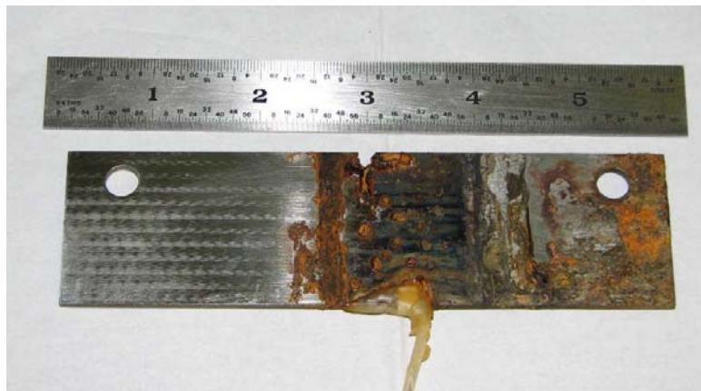
Figure 4. Photograph of corroded single edge crack specimen after being subjected to alternate immersion in a NaCl solution.
