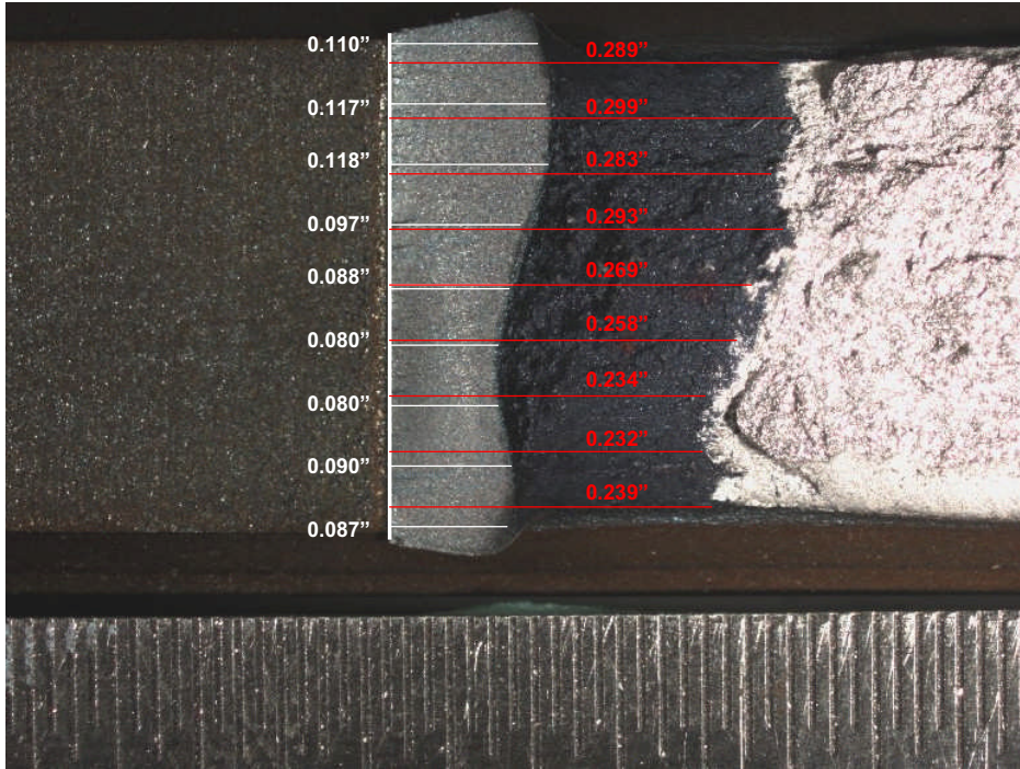
Figure A-3. Crack length measurements for specimen C1 (HAZ) of the flux-cored welded A516 steel
