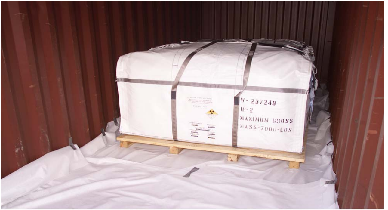
Figure G-4 Silo 3 Soft Sided Container Loaded into Shipping Container
