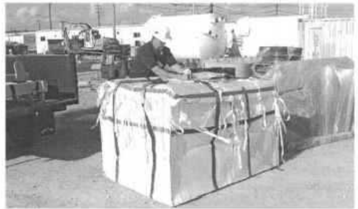
Representative DOT LSA-II lined, soft-sided container
