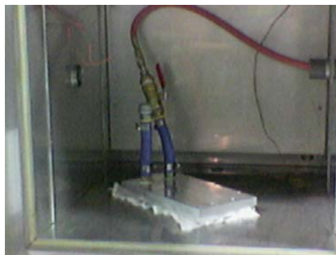
Figure 11. Baseplate leak test setup.
