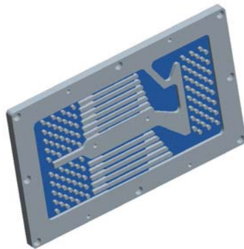
Figure 7. Alpha baseplate pin-fin design with pin-fin.
