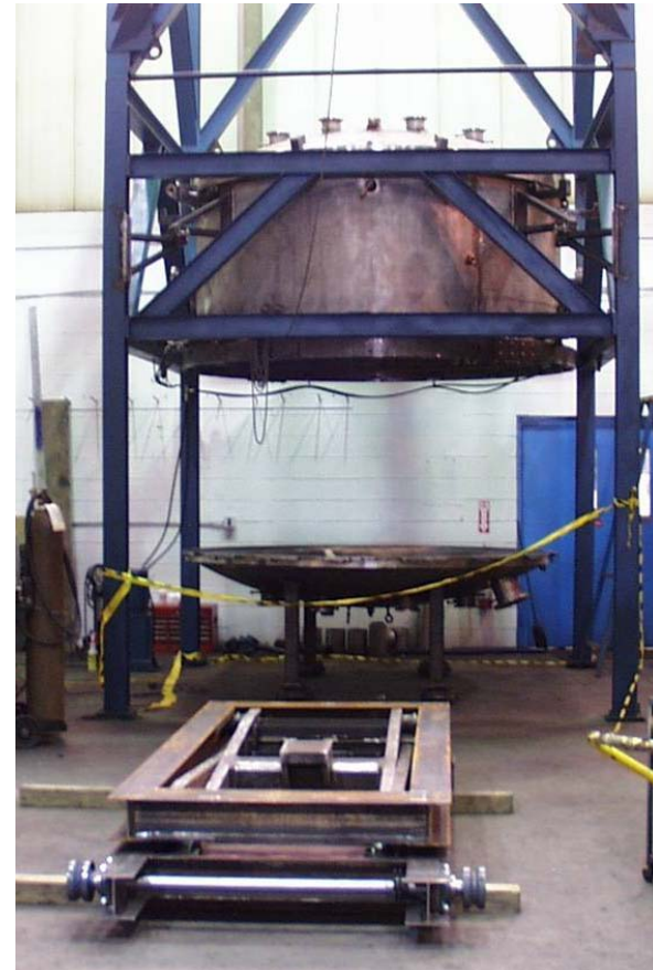
Silicon Carbide Substrate Furnace In Process (1.8 m diameter)
