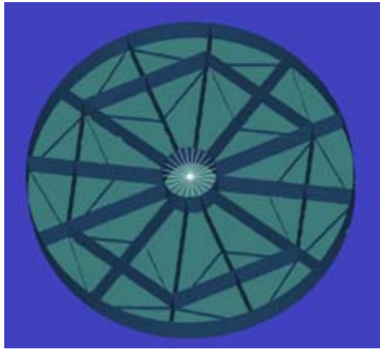
First Dynamic Mode (constrained) Frequency: 1811 Hz
