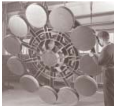
Right: Polishing wheels; using a molding machine to make bezels for window hand-crank; 1939 Deluxe Convertible Coupe.
