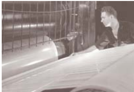
Right: Making fiber for tires. Woven cotton, dipped in molten rubber, is run through rollers to fuse and flatten the two materials.
