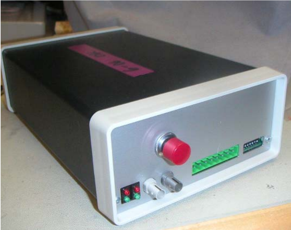
Figure 4A. ADCMOD, here version 3. Version 2 has a different power connector. The red button is for reboot of the firmware. Across the bottom are the indicator LED's, the fiber optics, the green terminal block for power/control of batteries, and (un-used) DIP switches.
