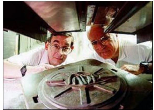
Drs. Dugan (l) and Jacobs view the underside of the LMR machine they developed to detect underground land mines for the U.S. Army. The technology is now being applied to find flaws in coatings and surfaces of the NASA Space Shuttle and its external fuel tanks.
