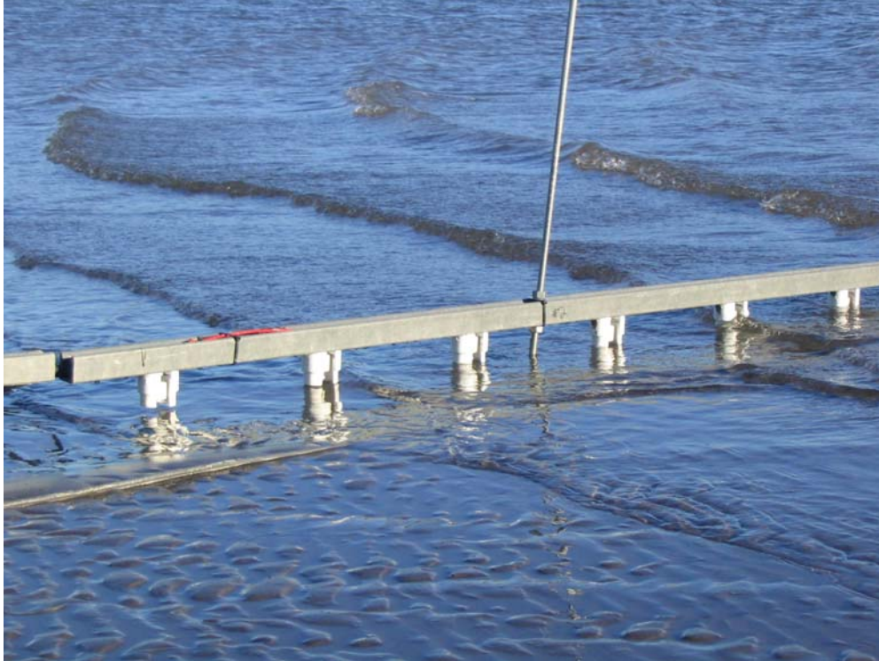
Figure A-9. Waves triggering floats on the wave run-up gage. The two floats at the right in the picture are activated in this photo.
