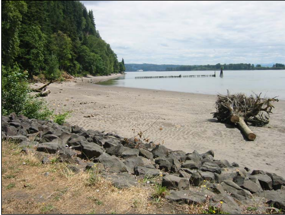
Figure A-1. County Line Park looking upstream. In addition to the large root wad, there are numerous local scour features around sloughed rip-rap.
