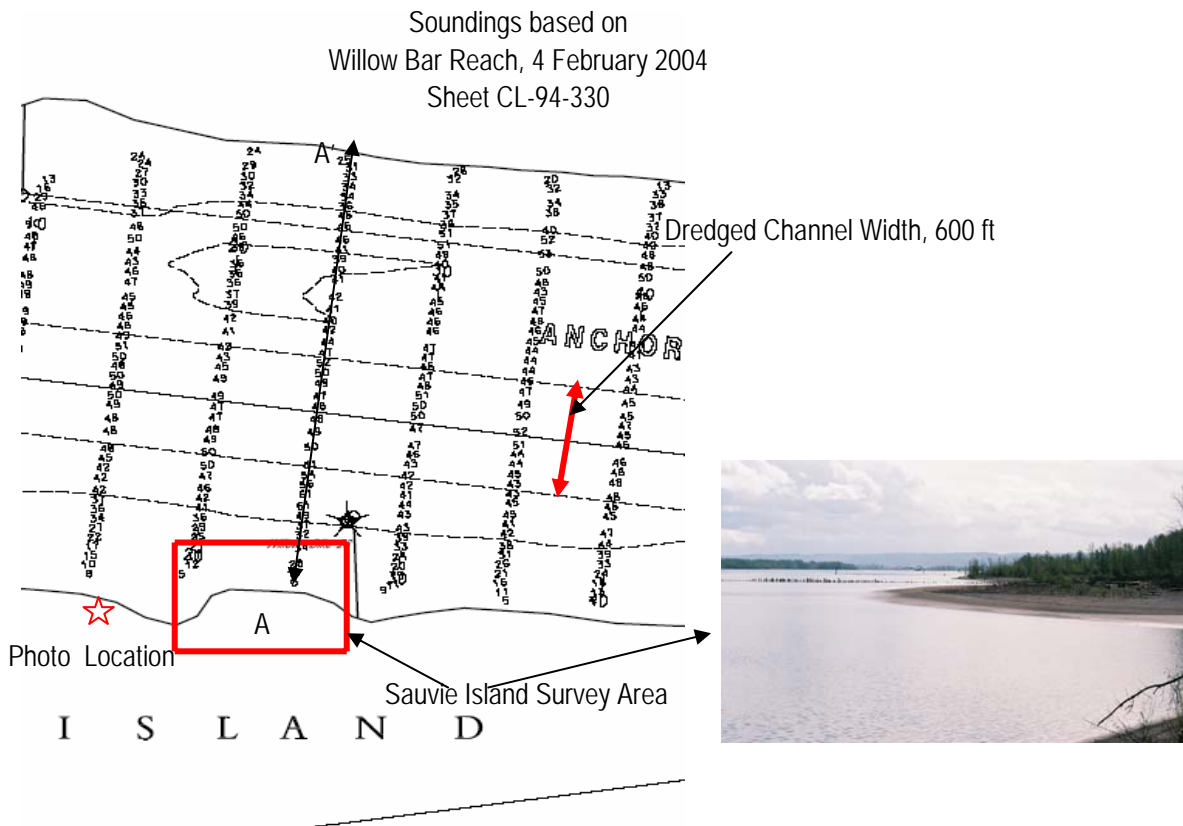
Figure 33. Willow Bar, Sauvie Island Survey Site. The channel cross-section A-A' was used in the NAVEFF calculations.
