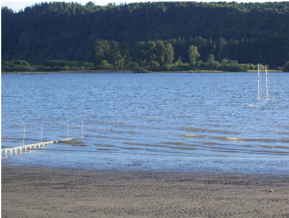
Figure A-10. Site layout, with wave run-up gage to left of photo and wave staff gages offshore to right of photo.
