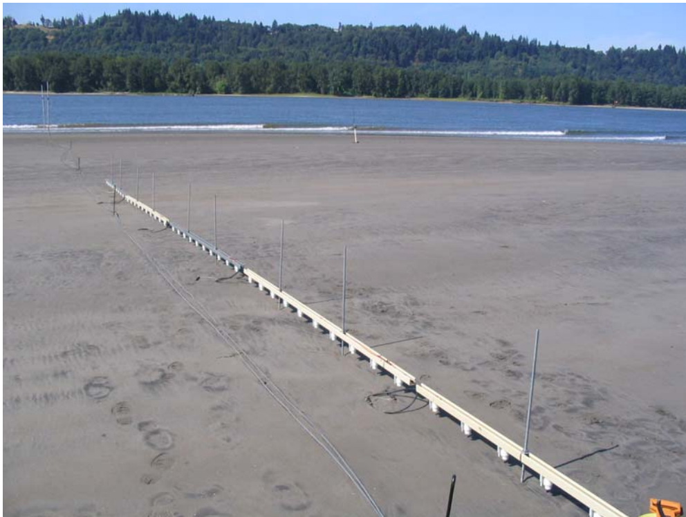
Figure A-8. Wave run-up gage, as installed at Barlow Point site
