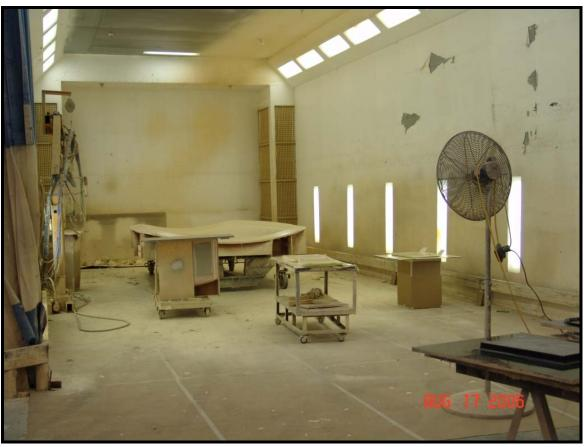
Figure 2: Gelcoat booth containing small part molds during the curing process
