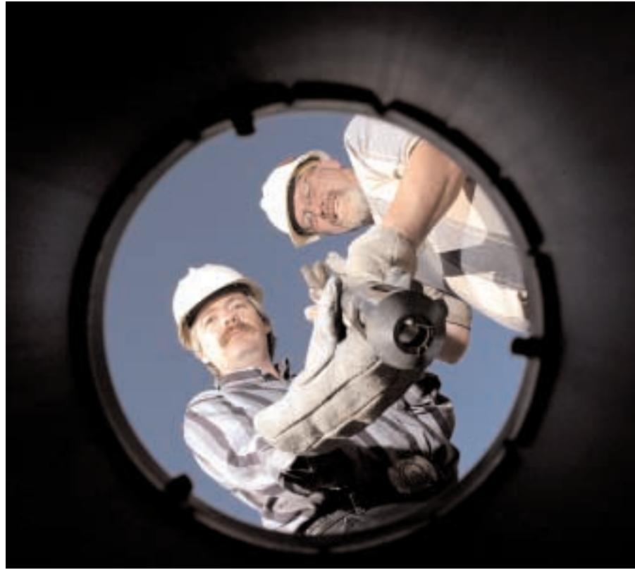
HOT STUFF — Joe Henfling, left, and Randy Normann (both 6211) show how their high-temperature electronics package can be lowered into a geothermal well. The package can function effectively at 250°C and more. (Photo by Randy Montoya)
