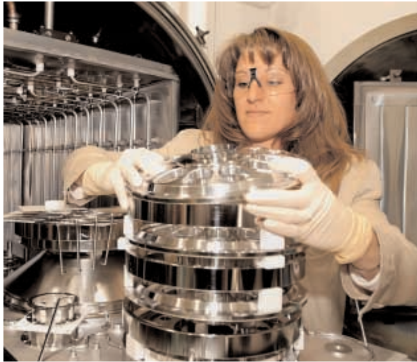
MARY WALKER (1670) uploads diode components into a hydrogen/vacuum firing furnace at the Z pulsed-power facility. Sandia's Materials Processing and Coatings Laboratory (MPCL) has received an ISO 9001 certificate of registration. (Photo by Randy Montoya)
