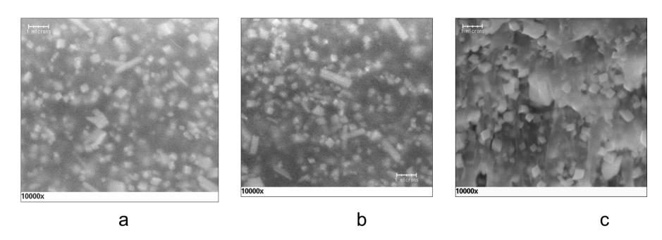
Fig. 2. SEM images of the new 60%  $H_3OZr_2(PO_4)_3$  / 40% PVDF(Si) membrane: (a) and (b) show the surface on the opposite sides of the membrane and (c) is the cross-sectional image.
