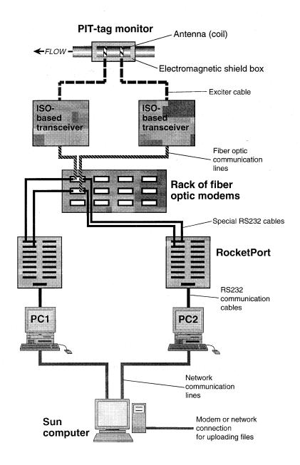
Figure 1. General schematic of a stationary 134.2-kHz ISO-based transceiver system that will be used at all Columbia River Basin dams in 2000.
