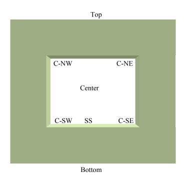
Figure 2. The figure depicts an insert-only style of antenna housing for orifices. It also shows some of the compass-based locations where measurements were taken to determine read ranges for PIT tags.
