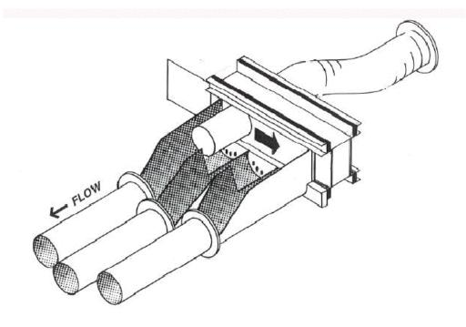
Figure 4. Diagram of a three-way side-to-side gate, a type of fish diversion gate.
